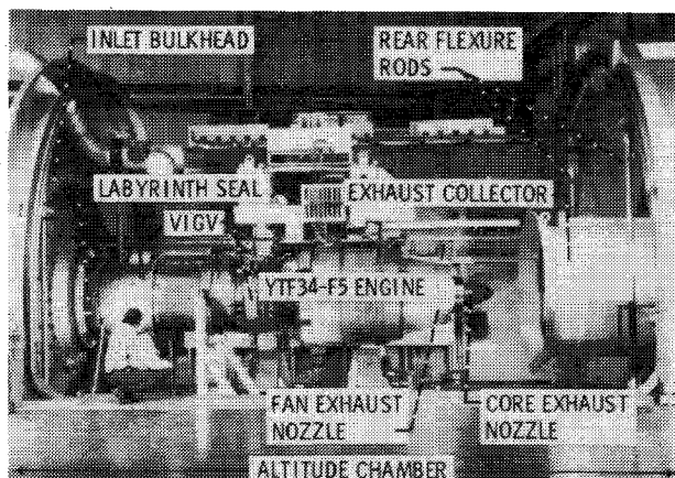
Fig. 1 TF-34 engine, with VIGV, installed in altitude facility.
